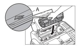
9 Insert the toner cartridge so that the guide (A) on the left side of the toner cartridge fits into the groove inside the machine and slide it down parallel to the guide.
